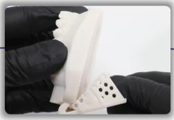
The supports on the bottom of each model can be easily removed by firmly holding the model and snapping the support plate away.
