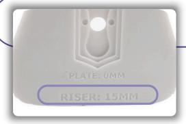
Each model will have a riser number printed on the bottom. This will correlate how many risers you will add to the corresponding upper or lower adapter.
