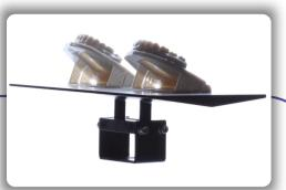
Print the upper and lower files. These files are already equipped with supports, so no additional supports are necessary. If your printer indicates otherwise, try a test print with the provided support before adding custom supports.
