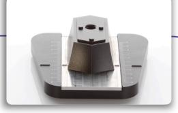
Place the upper and lower adapters on the articulator plates. Align the raised steel base lines to the raised plate lines at 0. Also, check that the front of the adapter base is flush with the edge of the articulator plate.
