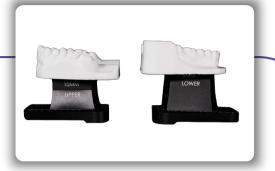
Secure each upper and lower model to the corresponding adapter. To do this, you will match the pins into the pattern on the 3D print.
