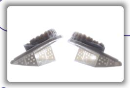
If additional supports are required, they should be placed on the bottom, avoiding the precision attachment pattern to prevent distortion.
